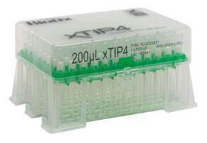
xTIP filter tips contain sintered polyethylene filters that deliver a secure barrier to block aerosol contaminants with a 99.99% bacterial filter efficiency.
