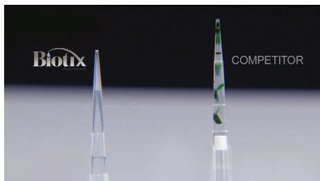
Figure 1 Biotix low retention pipette tip compared to a non-low retention pipette tip
